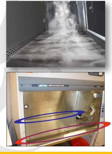
The laminar flow of air within the BSC prevents horizontal air mixing, but also produces airflow directed toward the user. Blockages in the front grill area create egress zones that can enable the release of aerosols into the room.
