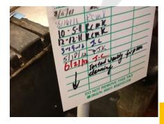
These flush/checks should be documented on attached eyewash tags or on log sheets kept in proximity to the eyewash fixture.
